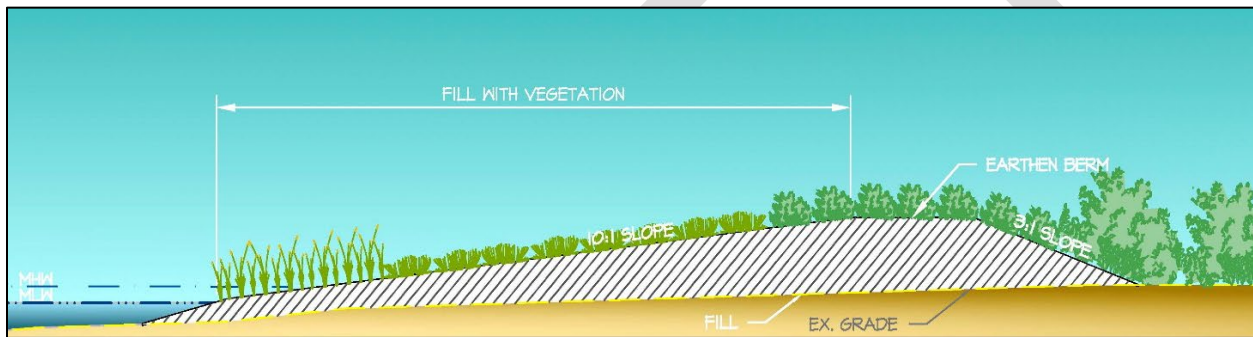
Figure 38 - New earthen berm with living shoreline
